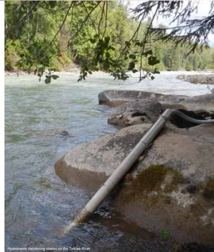
Hydrometric monitoring station on the Telkwa River
